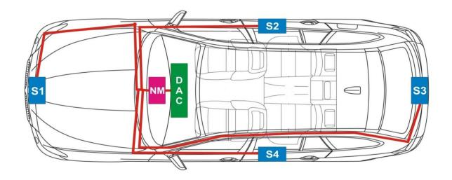
S1,S2,S3,S4 - Millimeter Wave Radar
